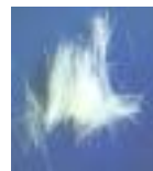
PVA :40.8 μm Lf:15.0mm
