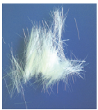
PVA① φ: 40.8 μm Lf: 15.0mm
